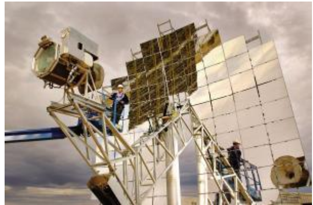
Sandia researcher Chuck Andraka makes adjustments to a Stirling Energy Systems, Inc. solar dish-engine system installed at Sandia's National Solar Test Facility earlier this year. Five more will be erected by January as test units. (Photo by Randy Montoya)
