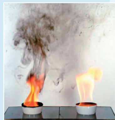
Synthetic fuel's combustion (on the right) is immensely cleaner than standard diesel's combustion (shown on the left)
